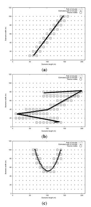
**Figure 2.** Illustration of the intruder tracking accuracy for different mobility patterns: (a) straight, (b) random and (c) curve.
