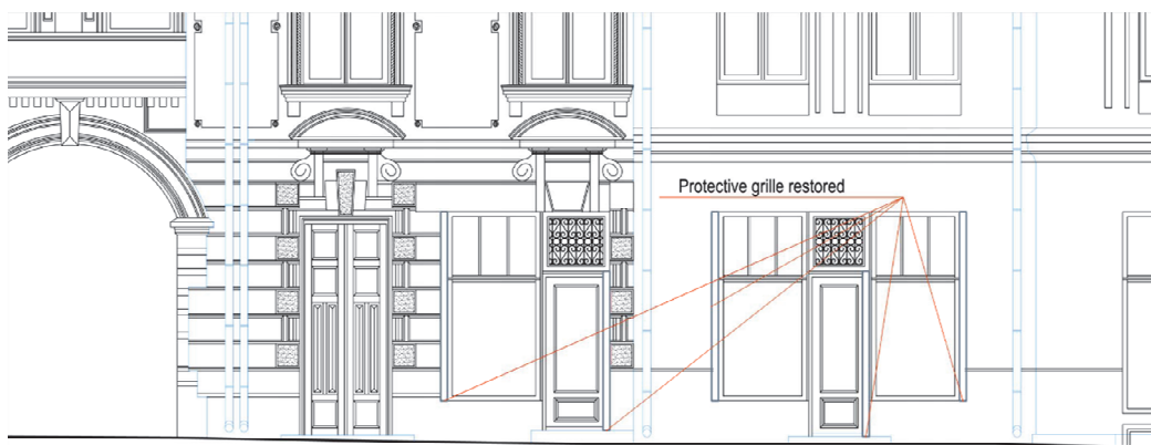
Figure 76. Demand of the protection grille for some access in the Facade draws
