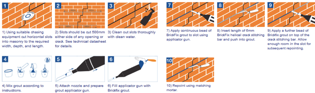
Figure 60. Process of Brickfix Crack Stitching System method
