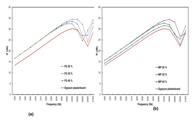
Fig. 4. Prediction of the acoustic isolation for MP and FG composites considered as an impermeable single-layer: (a) fiberglass, (b) mechanical pulp fibers. Comparison with gypsum plasterboard
