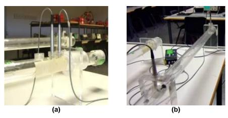
**Fig. 2.** Experimental equipments for measurement of (a) sound absorption coefficient (UNE EN ISO 10534-2:2004), and (b) the specific resistance to flow (Ingard & Dear method)
