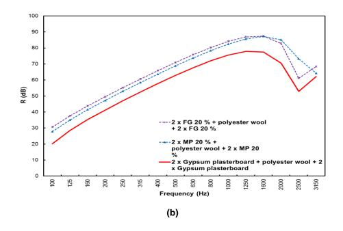
**Fig. 5.** Prediction of the acoustic isolation for double-layers of MP and FG composites: (a) without absorbing material, and (b) with absorbing material between the two layers
