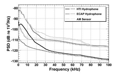
Figure 16. Power spectral density (PSD) of the noise level recorded in situ. Solid lines represent the median, dotted lines the 0.27% quantile (corresponding to a  $3\sigma$  deviation from the median). The voltage used is the calibrated input voltage of the AcouADC board.
