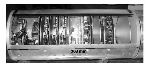
Figure 11. An LCM during assembly, equipped with AcouADC boards before insertion into the titanium container. The sockets for external connection (not visible in this picture) are attached to the lid of the container on the left-hand side of the photograph. From left to right, the following boards are installed: a Compass board; three AcouADC boards; a DAQ board; a Clock board.
