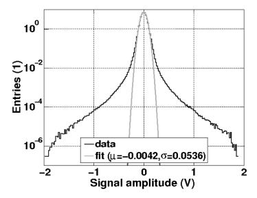
Figure 4. Normalised distribution of signal amplitudes for all data recorded with the AMADEUS-0 device. High amplitude (>2 V) signals, saturating the readout electronics, have been removed. A gaussian fit to the data yields mean  $\mu$  and standard deviation  $\sigma$ .
