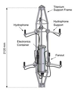
Figure 2. Drawing of a standard acoustic storey, or acoustic cluster, with hydrophones.
