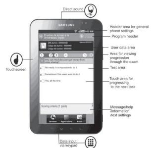
Figure 2. Functional structure of MM-PAU on Samsung Galaxy device.
