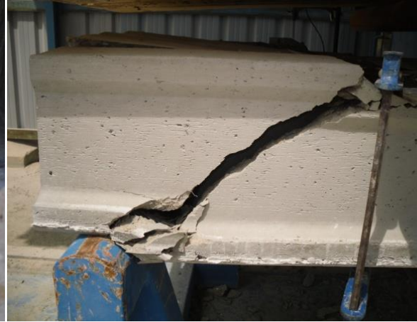
Fig. 9b. Crack caused by anchorage failure
