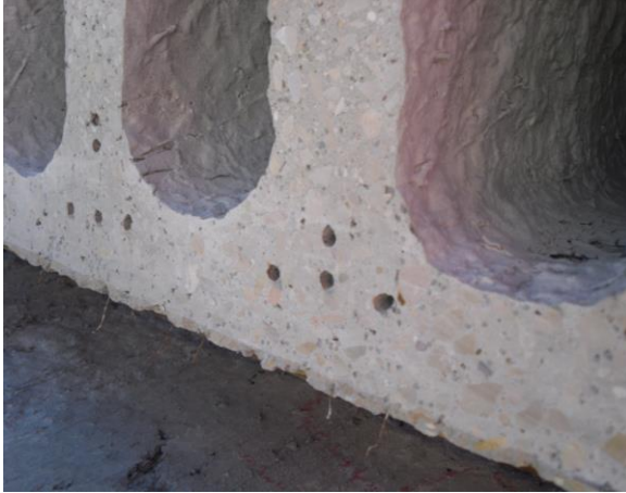
Fig. 9a. Sliding of the strands in concrete
