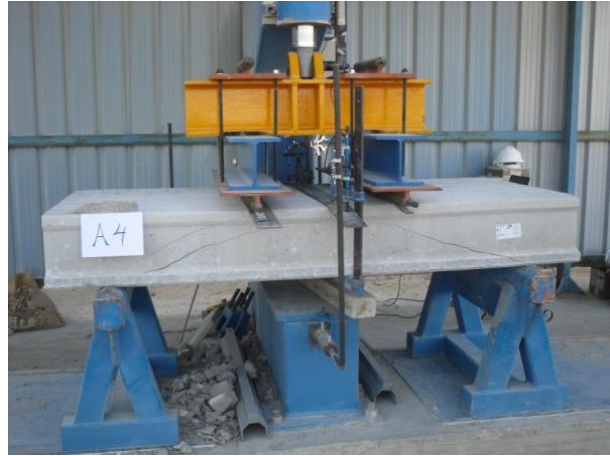
Fig.5. Test set-up. Shear diagonal tension failure
