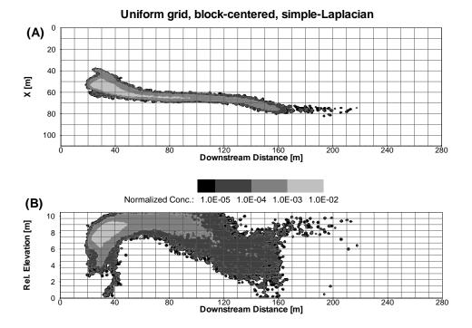
Figure 13: Transport at the coarse scale after upscaling the reference realization on a uniform grid using a block-centered simple-Laplacian approach for t = 328 days. (A) Depth-integrated normalized concentration distribution. (B) Laterally-integrated normalized concentration distribution.
