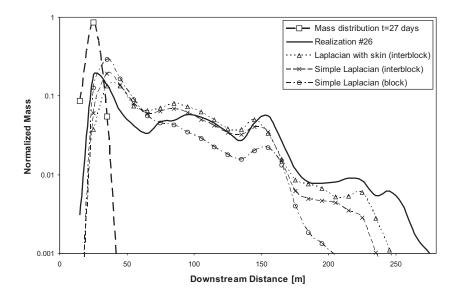
Figure 10: Longitudinal mass distribution profiles of the tritium plume from the fine scale reference realization, and predictions by some Laplacian-based upscaling approaches at the coarse scale, for t = 328 days.
