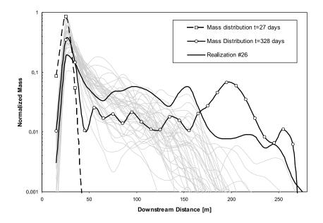
Figure 3: Longitudinal mass distribution profiles of the observed tritium plume at MADE, and predictions on several realizations of hydraulic conductivity. Each realization was generated (on natural-log space) over a grid of  $110 \times 280 \times 70$  cells by sequential Gaussian simulation using the variogram model in Equation 1.
