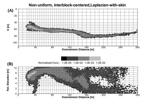
Figure 15: Transport at the coarse scale after upscaling the reference realization on a non-uniform grid using an interblockcentered Laplacian-with-skin approach for t = 328 days. (A) Depth-integrated normalized concentration distribution. (B) Laterally-integrated normalized concentration distribution.
