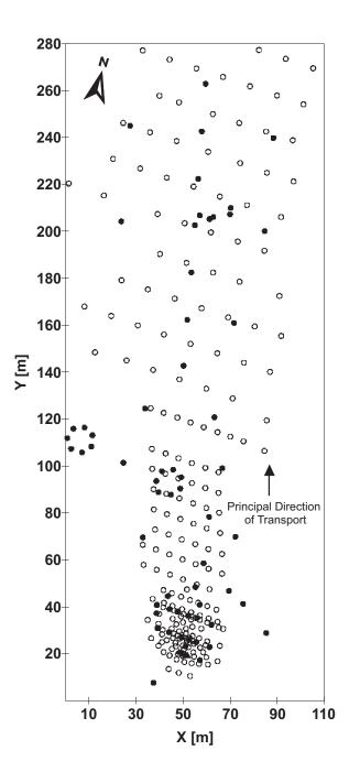
Figure 1: Plan view of model domain. Open circles denote multilevel sampler wells. Triangles indicate the tracer injection wells. Solid circles correspond to flowmeter well locations.
