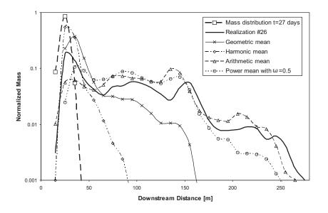
Figure 8: Longitudinal mass distribution profiles of the tritium plume from the fine scale reference realization, and predictions by some simple averaging upscaling approaches at the coarse scale for t = 328 days.
