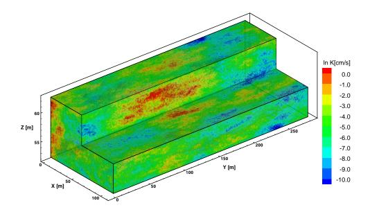
Figure 4: Realization #26 of  $\ln K$  from Salamon et al. (2007). This realization exhibits a strong solute tailing and it is used as the reference in the upscaling exercise. (The scale of the z-axis is exaggerated seven times for clarity.)
