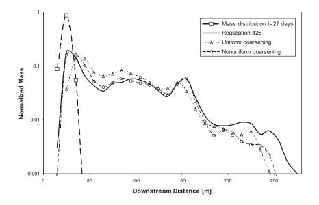
Figure 11: Longitudinal mass distribution profiles of the tritium plume from the fine scale reference realization, and predictions on uniform and non-uniform coarse scale grids, for t = 328 days.
