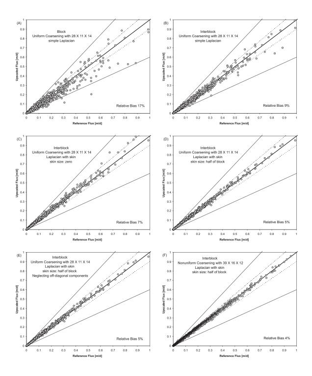
Figure 9: Flow comparison at the fine and coarse scales using Laplacian-based upscaling approaches. All circles within the dashed lines correspond to coarse scale values that deviate less than 10% from the reference ones; similarly, all circles within the outer solid lines correspond to coarse scale values that deviate less than 40%. The average relative bias, as defined in Equation 10, is reported in the lower right corner of each box.
