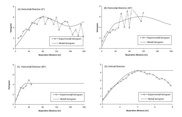
Figure 2: Horizontal and vertical experimental variograms, and fitted model, for the  $\ln K$  flowmeter data. The rotation angle of the directional variograms is measured in degrees clockwise from the positive *y*-axis.
