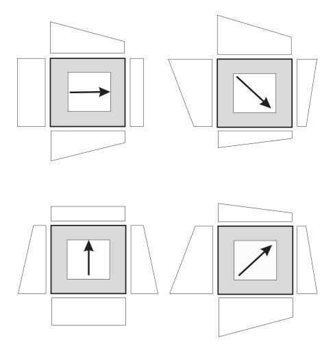
Figure 6: An example of four boundary condition sets that could be used in 2D for the local flow models when performing the Laplacian-with-skin upscaling. The white area is the block being upscaled, and the gray area is the skin region; the arrows indicate the (negative) mean head gradient induced by the prescribed head boundary conditions, and the shapes on the sides of the block indicate the magnitude of the prescribed heads given by tilting planes with gradients opposite to the arrows.
