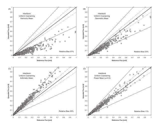
Figure 7: Flow comparison at the fine and coarse scales using simple averaging upscaling approaches. All circles within the dashed lines correspond to coarse scale values that deviate less than 10% from the reference ones; similarly, all circles within the outer solid lines correspond to coarse scale values that deviate less than 40%. The average relative bias, as defined in Equation 10, is reported in the lower right corner of each box.
