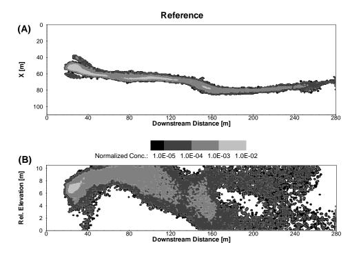
Figure 12: Transport in the fine scale reference realization for t = 328 days. (A) Depth-integrated normalized concentration distribution. (B) Laterally-integrated normalized concentration distribution.
