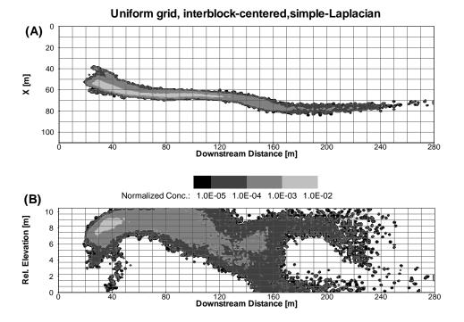
Figure 14: Transport at the coarse scale after upscaling the reference realization on a uniform grid using an interblock-centered simple-Laplacian approach for t = 328 days. (A) Depth-integrated normalized concentration distribution. (B) Laterally-integrated normalized concentration distribution.
