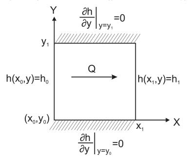
Figure 5: Boundary conditions that would be used in 2D for the local flow model when performing the simple-Laplacian upscaling in order to determine the *x*-component of the hydraulic conductivity tensor. In the simple-Laplacian approach, it is always assumed that the principal directions of the conductivity tensor are parallel to the reference axes.
