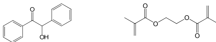
Figure 1.3: Chemical structure of the initiator benzoin (left), and the crosslinker EGDMA (right).
