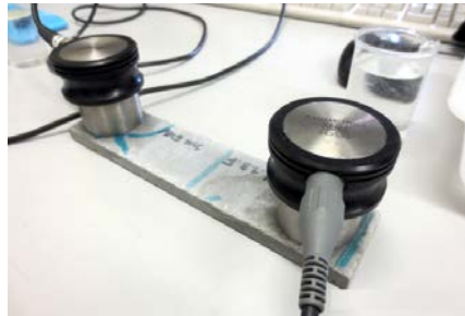
Figure 5. Test setup for UGW experiments
