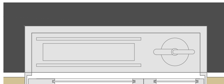
BIE 25mm + extintor 21A-113B detalles E; 1/20
