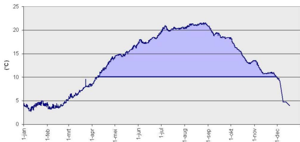
Figure 6.2. Seasonal temperature variation in drinking water in Diemen. The period when heat recovery is possible is shown in blue.
