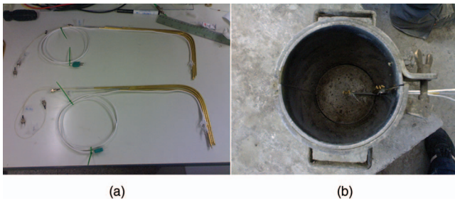
Fig. 3 (a) Two sets of sensors fabricated. (b) Location of these sets inside the cylindrical mold before concrete pouring.
