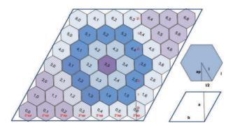
Figure 4: Final shape of the work area made up of hexagonal cells throughout which the mobile nodes are distributed.
