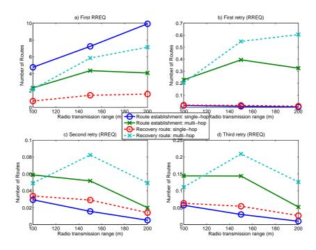
Figure 14: Number of routes found or recovered for each route request packet with an error rate of 1%, an average node movement speed of 1.38 m/s and a session time of 180 s. Single-hop and multi-hop routes found according to search attempt.
