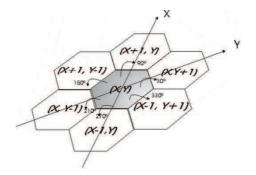
Figure 3: Work area formed with hexagonal cells. Depending on the starting cell and on the angle of movement of the node we obtain the coordinates of the destination cell.
