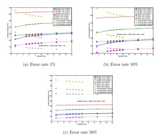
Figure 13: Percentages of single-hop, multi-hop and unreachable communications for different radio transmission range values. Session time 180 s, error rates of 1%, 10%, and 50%, and different node movement speeds.
