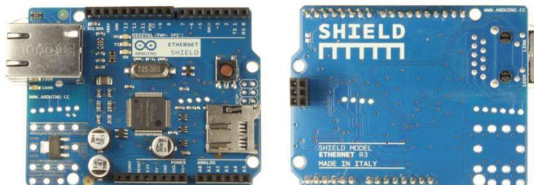
**Figura 5. Vista frontal y trasera Ethernet Shield [1]**
