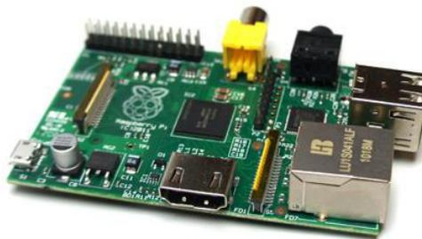
Figura 14: Vista Raspberry Pi (modelo B) [13]
