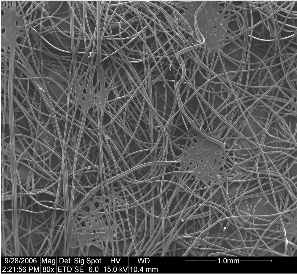
Figure 4.- SEM microphotograph (80x) of the polypropylene nonwoven substrate collector as received without any surface treatment. 541x499mm (96 x 96 DPI)
