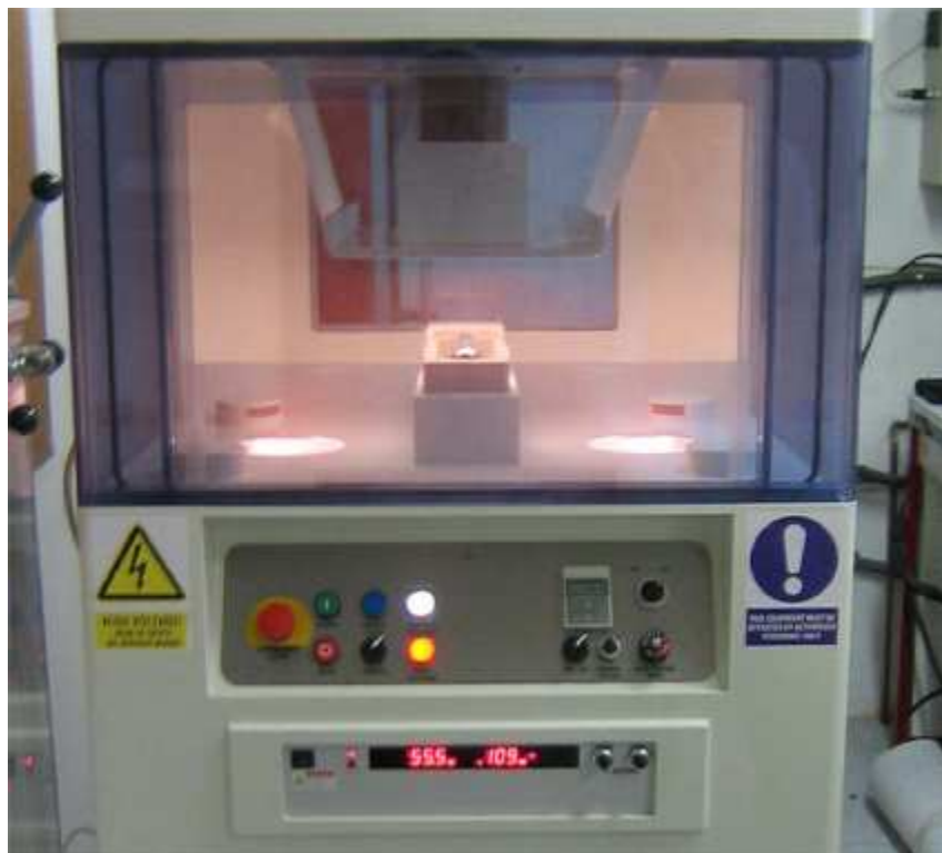
Figure 1.- Representation of the Nanospider TM electrospinning equipment, a) schematic representation, b) photograph of the Nanospider TM apparatus. 149x134mm (72 x 72 DPI)
