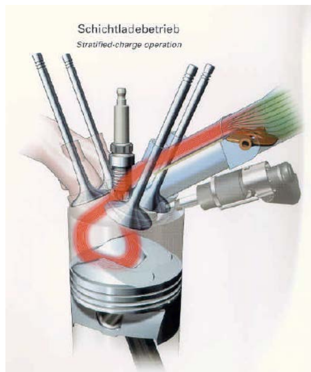
Figure 6-37: FSI concept – description of the stratified mode [6-19]
