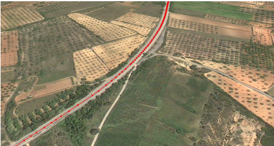
Figure 116. Example of how the polyline is created. Notice the higher density on the horizontal curve.
