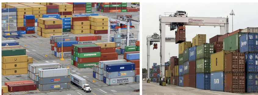
Figure 2: A container yard (left) and gantry cranes (right) (Photos by Stephen Berend)
