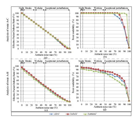
Figure 10: Experimental results after applying the link-quality-based packet replication.
