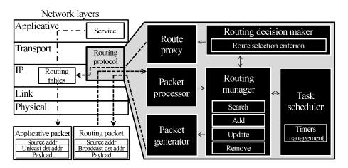
Figure 2: General architecture of a proactive routing protocol.
