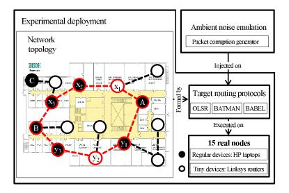
Figure 4: Experimental WMN deployment.
