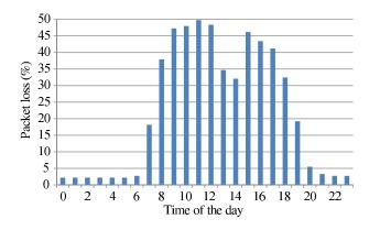
Figure 3: Packet loss conditions in the considered indoors scenario.
