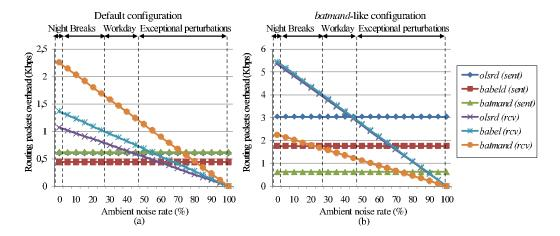
Figure 7: Routing overhead induced by routing packets sent and received.
