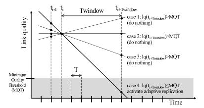
Figure 8: Link-quality-based adaptive packet replication technique.
