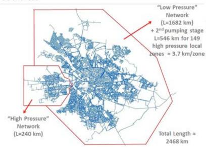
Figure 3: Anatomy of the water distribution system in Bucharest (Apa Nova, 2013)
