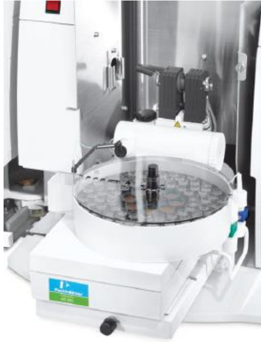
Figura 29. Automuestreador AS 900 PerkinElmer [92].
