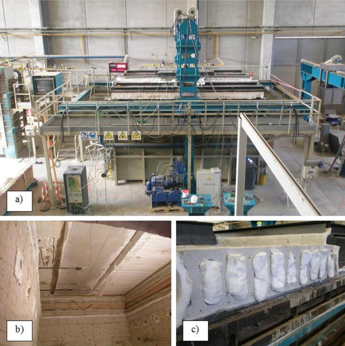
Figure 2. a) General view of the experimental setup. b) Inside the furnace. c) HC infilling
