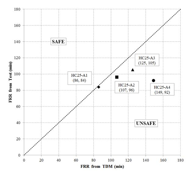
Figure 15. Comparison of Tabulated Data Method with test results
