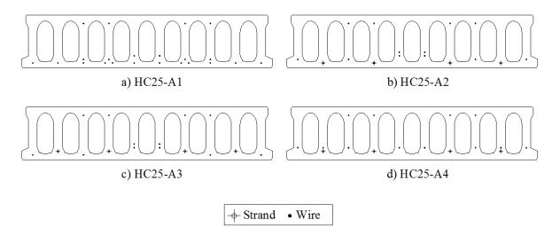
Figure 1. Cross-section and reinforcement arrangement of the HC slabs tested
