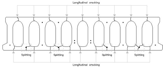
Figure 8. Crack patterns: a) Wire reinforcement. b) Wire/strand reinforcement
