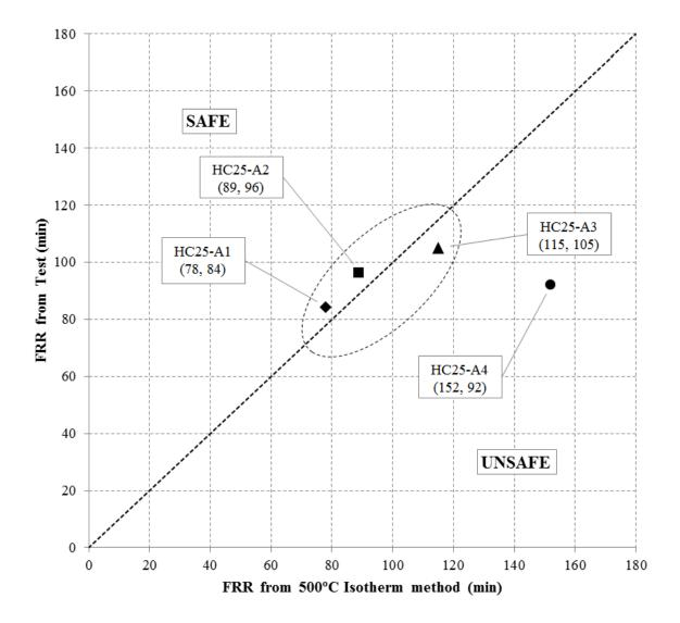
Figure 17. Expected FRR from 500°C Isotherm Method versus FRR measured in tests
