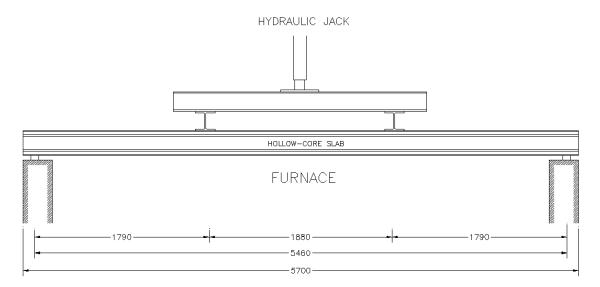
Figure 3. Representation of the experimental setup.
