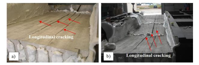
Figure 7.General view after the test. a) Longitudinal cracking of unit HC25-A1. b) Longitudinal cracking of unit HC25-A1.
