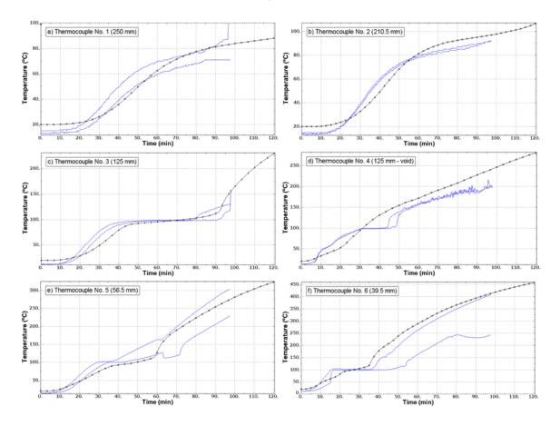
Figure 14. Comparison of measured temperatures for slab HC25-A2 calculated using the numerical model (dotted line).
