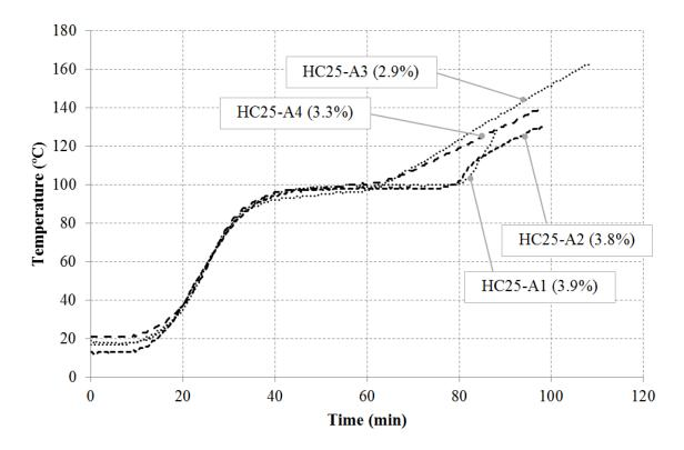
Figure 12. Influence of moisture content. Comparison of thermocouple number 3, located 125 mm from the exposed surface in each slab.
