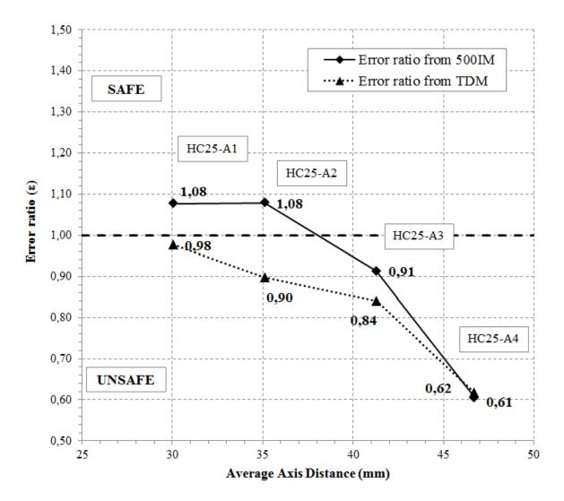
Figure 18. Average axis distance versus error ratio from both Tabulated Data Method and 500°C Isotherm Method.
