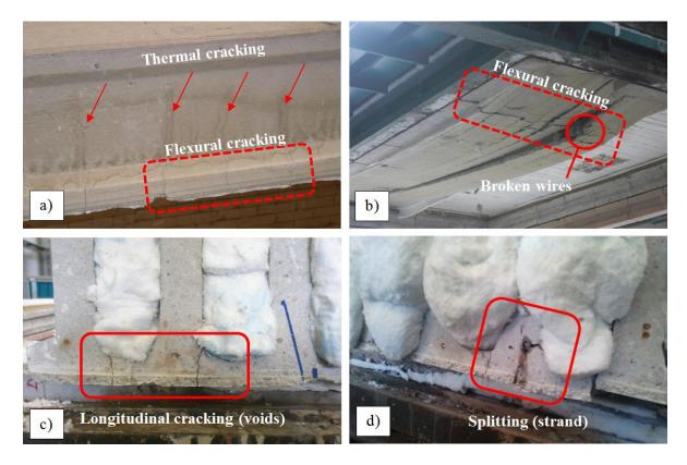
Figure 6. Cracking types: a) Thermal cracking in the web and flexural cracking (HC25-A2). b) Flexural cracking and broken wires from below (HC25-A1). c) Longitudinal cracks through the bottom flange (HC25-A2). d) Splitting around one strand of the HC25-A3
