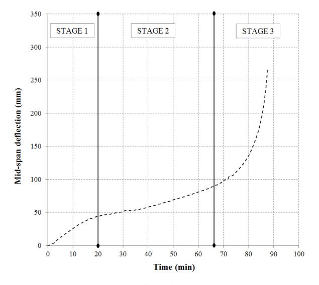
Figure 9. Time versus mid-span deflection. Identification of each stage
