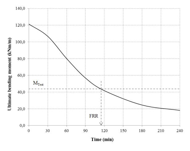
Figure 16. Time of exposure versus ultimate bending moment from the 500°C Isotherm Method for obtaining FRR.
