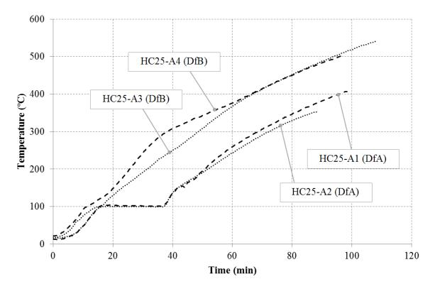
Figure 13. Temperatures at 39.5 mm from the exposed surface of each slab (Thermocouple number 6). DfA stands for Drilled from Above while DfB stands for Drilled from Below.
