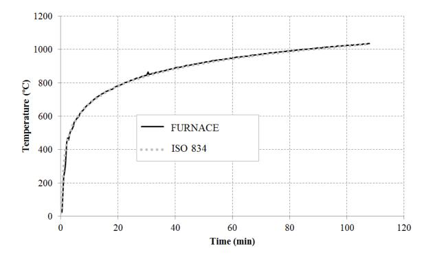
Figure 11. Comparison of the gas temperature inside the furnace with standard fire curve ISO 834
