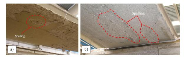
Figure 5. Spalling on the bottom surface of unit HC25-A2: a) Central zone. b) Support zone.
