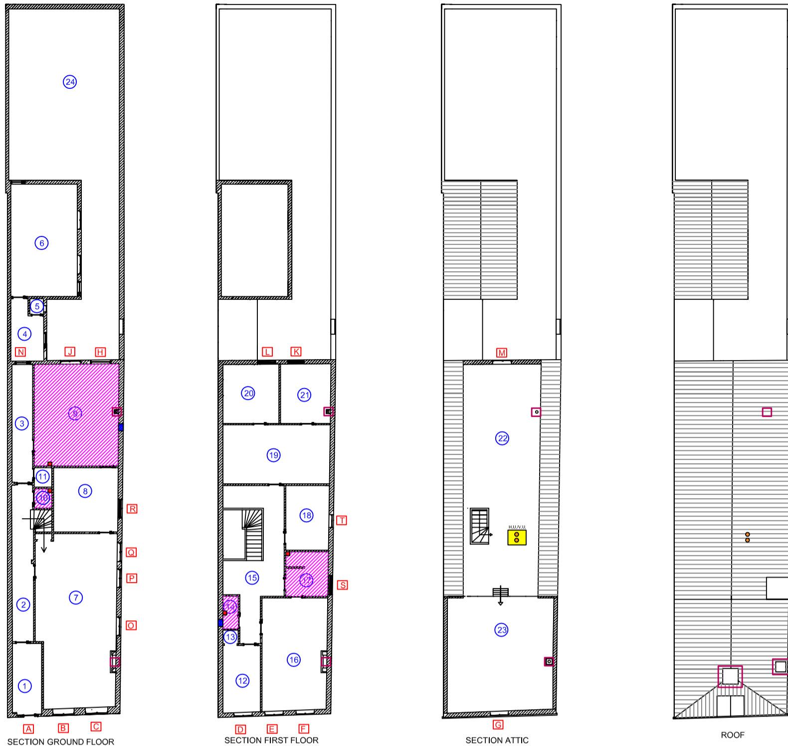
Distribution of the existing ventilation inside the building. Scale 1:250
