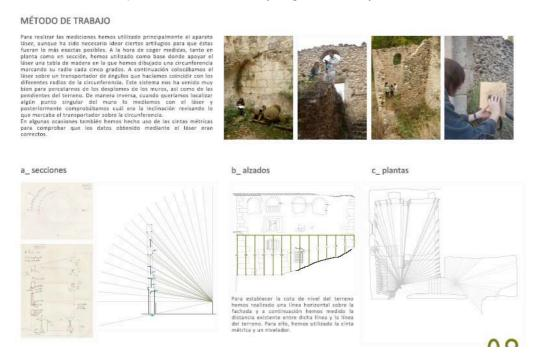
Fig. 2. Methodology used for the graphical survey of the building. Practical work developed during the course 2010-2011 (Authors: L. Cambra, L. Gilabert, J.E. Gómez, S. Sanchís)
