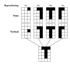
Figure 1. Example of transformation of a  $4 \times 5$  binary image into a sequence of four 15-dimensional binary feature vectors  $O = (\mathbf{o}_1, \mathbf{o}_2, \mathbf{o}_3, \mathbf{o}_4)$  using a window of width 3. No repositioning (top) is compared with the vertical repositioning (bottom).
