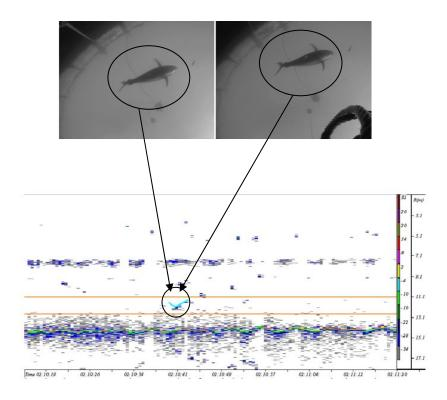
**Figure 2**. Images taken by the two camera system VICASS (left and right, respectively) and traces found at the instant in time at which images are made marked in the echogram. (22/01/2010 at 15:10:40 day hours. Mean TS is -29.3 dB and the distance to the center of gravity of the transducer is 12.1 m)
