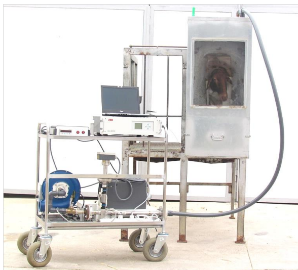
Figure 2.1. Whole mobile open-circuit respirometry system. Head hood attached to the front structure of a double metabolic cage with an animal on it.
