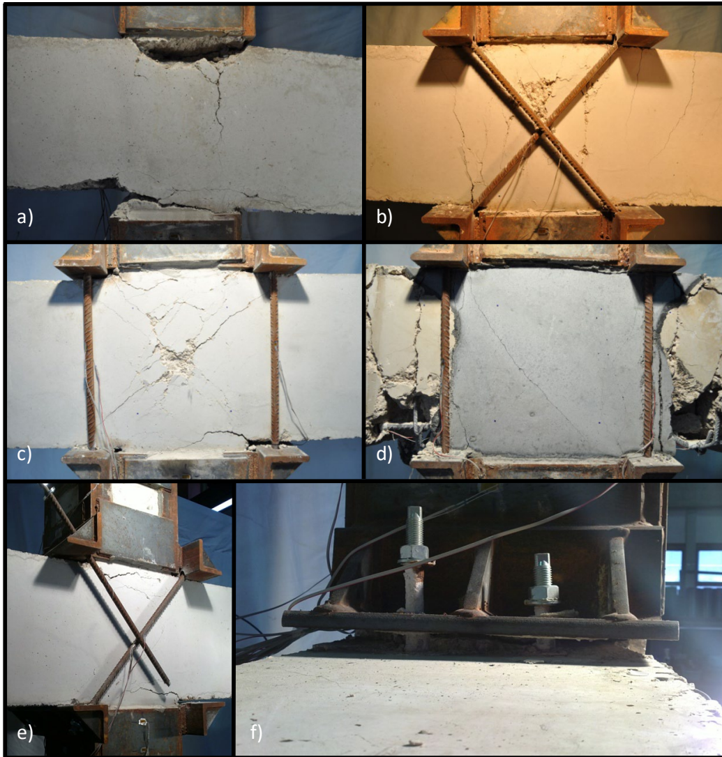
Figure 13. Photographs of principal failure modes. a) Bending failure in column-joint connections (specimen A.W.L0-2), b) Positive and negative bending failure in beams (specimen A.DB.L1-1), c) Shear failure in joint (specimen VB.L0-1), d) Failure transferred to beams after repair (specimen A.VB.L1-R), e) Tensile failure of external bars (specimen S.DB.L0-1), f) Pull-out failure of chemical anchor (specimen A.CA.L0-2)
