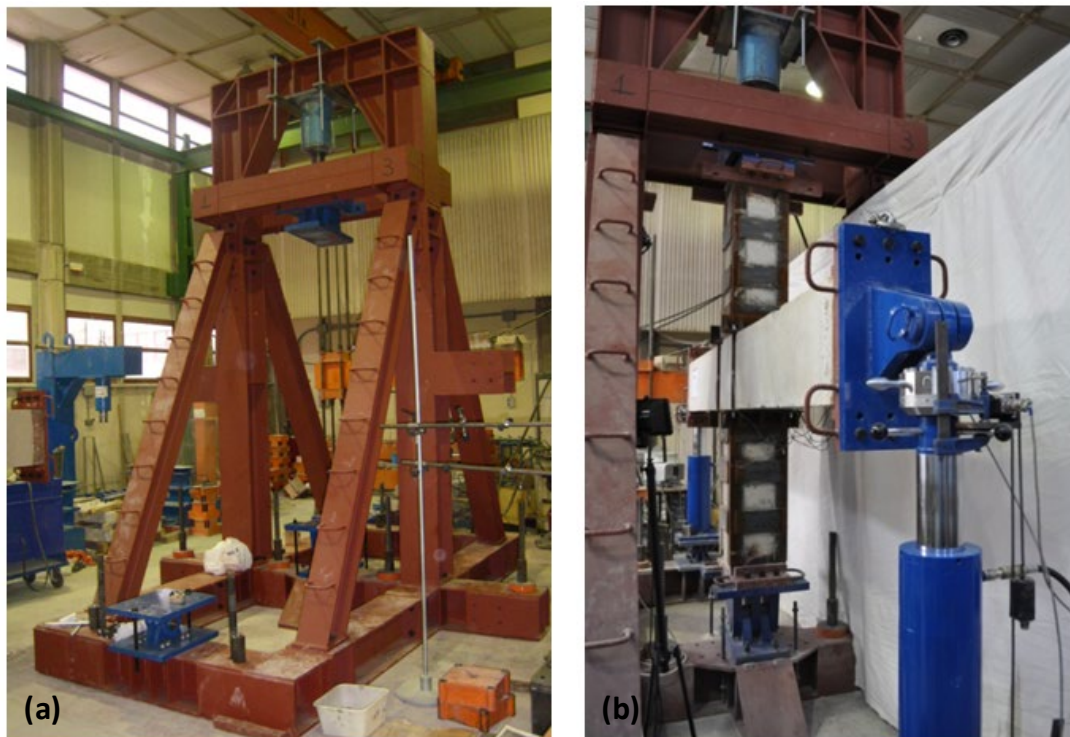
Figure 8. a) Frame attached to floor, b) Specimen set-up ready for test
