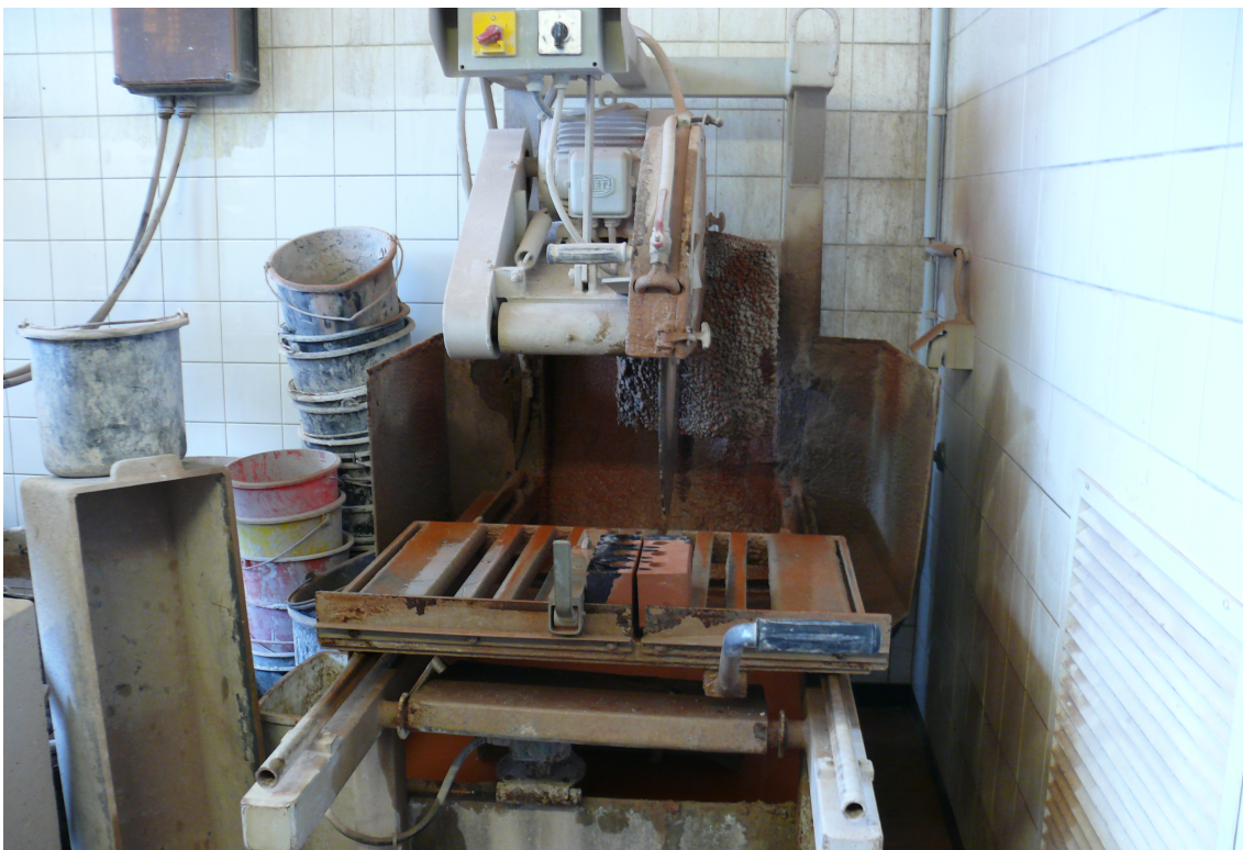
Pic. 3.3.2.1 Cutting bricks
