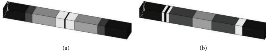
FIGURE 2: FE of the sleeper cracked at its central section (a) and at rail-seat section (b).
