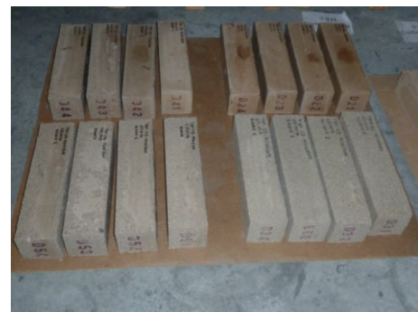
FIGURE 6: Specimens used for the flexural strength.
