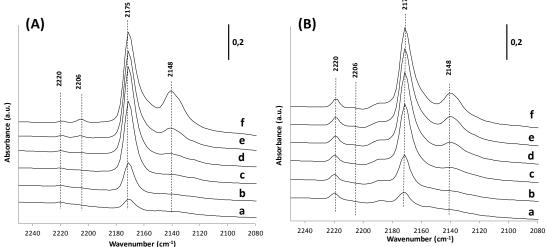
Figure 15: FTIR spectra of NO adsorbed at -175°C on calcined Cu-9 (A) and after being aged at 750°C during 13 hours (B). Each sample has been measured at increasing NO pressures: 0.10-0.12 (a), 0.20-0.23 (b), 0.28-0.31 (c), 0.45-0.51 (d), and 0.57-0.62 mbar
