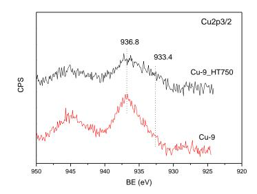
Figure 13: Cu2p<sub>3/2</sub> XPS line of the Cu-9 and Cu-9\_HT750 samples
