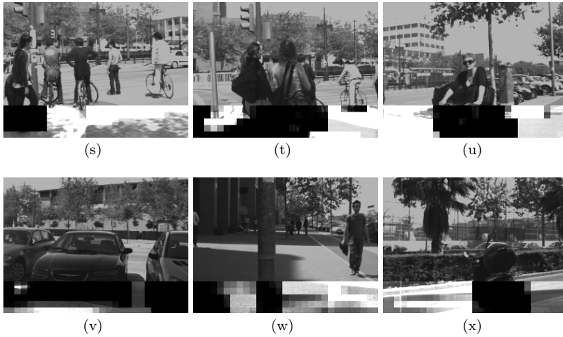
Fig. 7 Processed testing set, where brighter areas show detected free paths. Darker areas indicate a smaller certainty to be part of an obstacle-free area.
