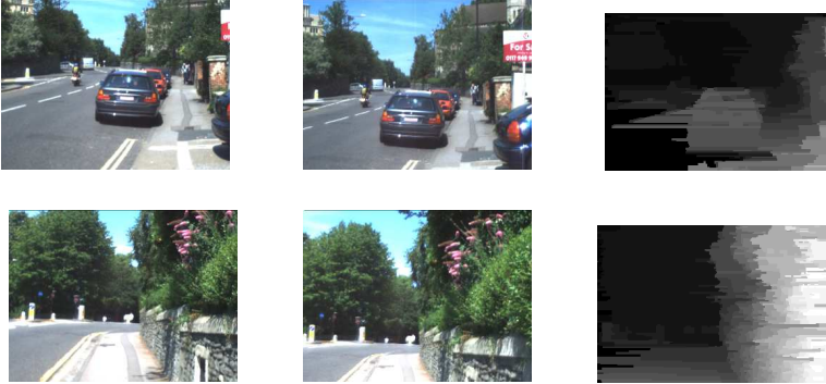
Fig. 1 Examples of stereo images before rectification and disparity maps. Left and right images are shown in first and second columns respectively and third column shows the corresponding disparity maps computed using the reference chosen.
