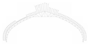
Figure 3. External pressure coefficients for lateral wind.
