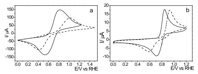
**Figure 4:** Stabilized cyclic voltammograms of glassy carbon electrodes (GC, dashed lines) or glassy carbon electrodes modified with single walled carbon nanotubes incorporated into silica layers (GC/SWCNT@SiO<sub>2</sub>, solid lines). Test solutions: (**a**) 0.5 M H<sub>2</sub>SO<sub>4</sub> + 10 mM iron (II) sulfate/ 10 mM iron (III) sulfate solution and (**b**): 0.5 M H<sub>2</sub>SO<sub>4</sub> + 1mM dopamine solution; scan rate: 50 mV/s; electrode geometric area: 0.07 cm<sup>2</sup>.
