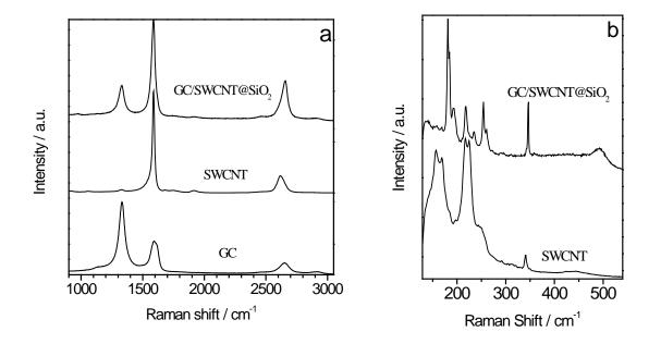
**Figure 3:** Raman spectra recorded (a) in the full frequency range and (b) RBM frequency region for: Bare glassy carbon electrode (labelled as GC), SWCNT powder from a DMF suspension (labelled as SWCNT) and SWCNT@SiO<sub>2</sub> prepared by electroassisted deposition deposited on a GC electrode (labelled as GC/SWCNT@SiO<sub>2</sub>).
