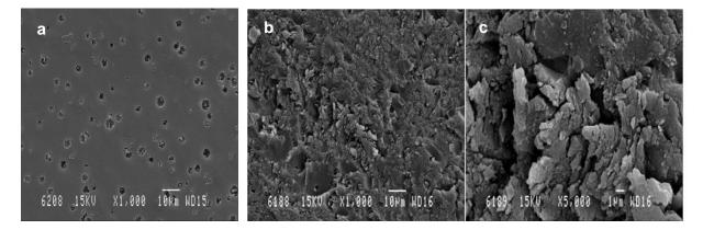
**Figure 1:** SEM micrographs acquired at different magnifications from: a) bare glassy carbon electrode, b) and c) glassy carbon substrate after the electroassisted deposition of the SWCNT@SiO<sub>2</sub> composite.
