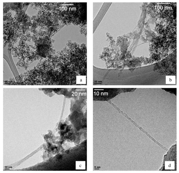
**Figure 2**. TEM micrographs of SWCNT@SiO<sub>2</sub> composites prepared by electroassisted deposition. (a) General view of the SWCNT@SiO<sub>2</sub> composite; (b) and (c) details of nanotubes bundles; (d) isolated SWNT found in-between SiO<sub>2</sub> aggregates.
