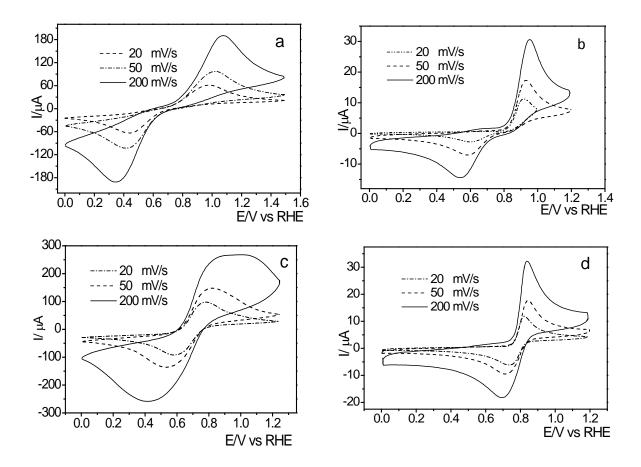
**Figure 5:** Steady state cyclic voltammograms recorded at different scan rates for: a) GC in 0.5 M  $H_2SO_4 + 10$  mM iron (II) sulfate/ 10 mM iron (III) sulfate solution; b) GC in 0.5 M  $H_2SO_4 + 1$  mM dopamine solution. c) GC/SWCNT@SiO<sub>2</sub> in 0.5 M  $H_2SO_4 + 10$  mM iron (II) sulfate/ 10 mM iron (III) sulfate solution; d) GC/SWCNT@SiO<sub>2</sub> in 0.5 M  $H_2SO_4 + 1$  mM dopamine solution. Electrode geometric area: 0.07 cm<sup>2</sup> in all cases.
