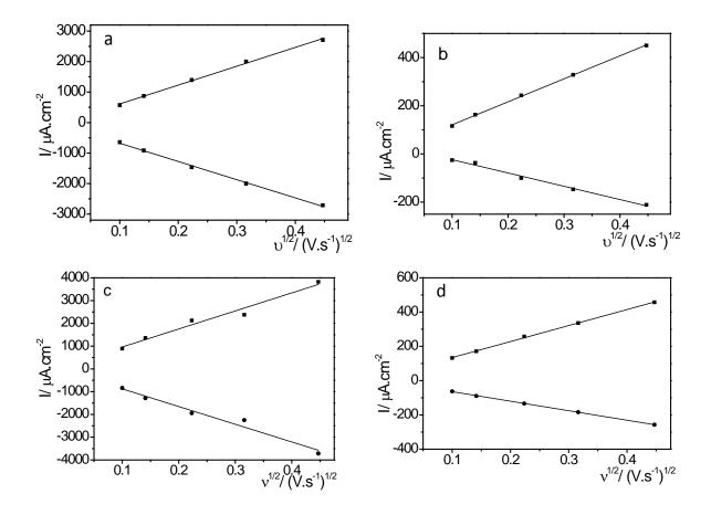
**Figure 6:** Randles-Sevcik plots obtained from voltammetric data for: a) GC in 10 mM  $Fe^{2+}/Fe^{3+}$  solution; b) GC in 1 mM dopamine solution; c) GC/ SWCNT@SiO<sub>2</sub> in 10 mM  $Fe^{2+}/Fe^{3+}$  solution; d) GC/SWCNT@SiO<sub>2</sub> in 1 mM dopamine solution. Electrode geometric area: 0.07 cm<sup>2</sup> in all cases.
