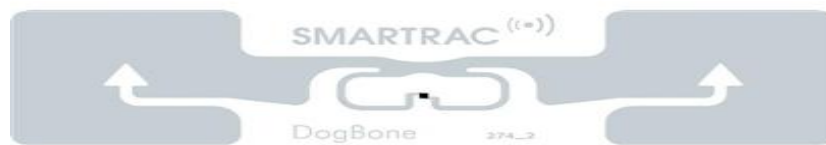
Figure 4. RFID UHF 2 GEN chip tag.
