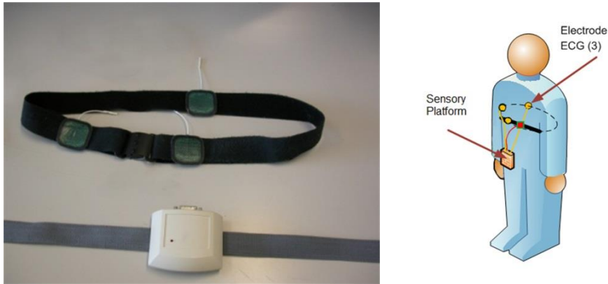
Figure 4.7. Illustration of R-TIPS. This platform allows wireless monitoring of cardiac signals. (a) It consists of a transmitter system and three sensors. (b) The transmitter system is placed on the participant's hip, and the sensors are placed below right breast, on the right side, and on the back.
