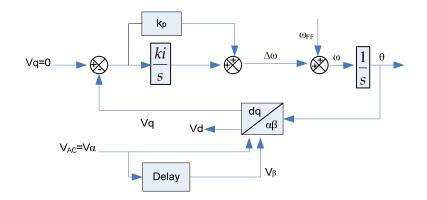
Fig. 3. Block diagram of the dqPLL.
