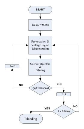
Fig. 8 Algorithm of the proposed islanding detection method.
