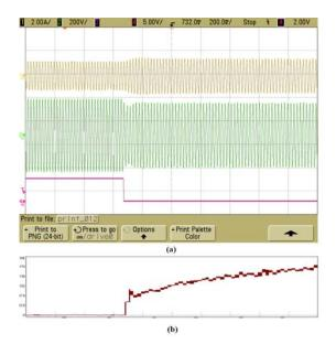
Fig. 15. (a) System behavior in islanding situation without disconnection, with RLC load. Up: inverter output current, 2 A/div.
