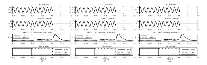
Fig. 10 Simulation results with R load. (a) ideal purely sinusoidal grid voltage. (b) grid voltage with a 5% third harmonic distortion.
