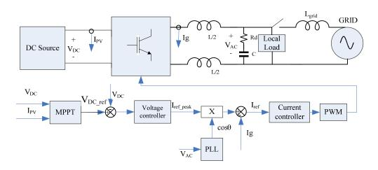
Fig. 2. Block diagram of the inverter.
