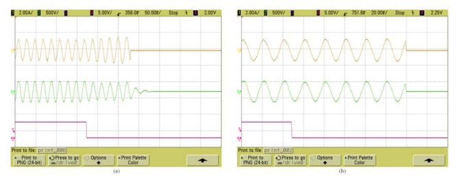
Fig. 16 Experimental results. (a) RLC Load. Up: inverter output current, 2 A/div. Center: Voltage at the local load, 500 V/div. Down: Grid disconnection signal, 5 V/div. Time scale: 50 ms/div. (b) R Load. Up: inverter output current, 2 A/div. Center: Voltage at the local load, 500 V/div. Down: Grid disconnection signal, 5 V/div. Time scale: 20 ms/div.
