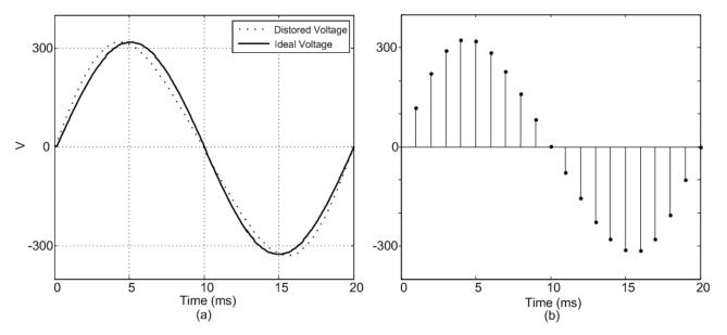
Fig. 6(a) Output voltage (ideal and distorted), (b) Discretized distorted voltage signal
