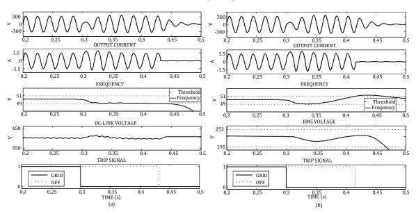
Fig. 13 Simulation results with RLC load. (a) SFS Method (*Kf=8*). (b) GEFS Method.
