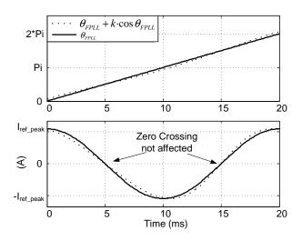
Fig. 5. Up: Ideal,  $\theta_{FPLL}$ , and distorted,  $\theta_{INV}$ , output phase waveform of the PLL. Low: ideal and distorted output current reference,  $I_{ref}$ ,
