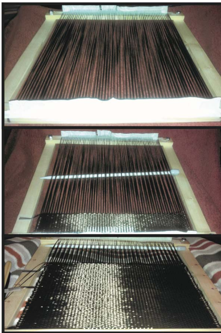
Figure 1. Photograph of the manufacturing process of slate plain fabrics by using a hand loom.
