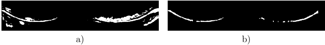
Figure 9: a) OR operation of three consecutive thresholded projections; b) Set of inliers or a quadratic distribution filtered with RANSAC.
