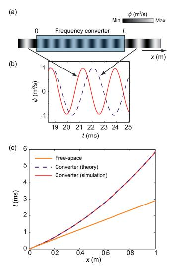
FIG. 2. Acoustic frequency converter designed with ATA. (a) Velocity potential as a function of space at a given instant. (b) Time dependence of the velocity potential at two different positions to the left and right of the converter. (c) Trajectory followed by an acoustic ray inside a converter with  $a = 1 \text{ m}^{-1}$ .
