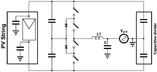
Fig. 12. The NPC half-bridge with capacitive divider.
