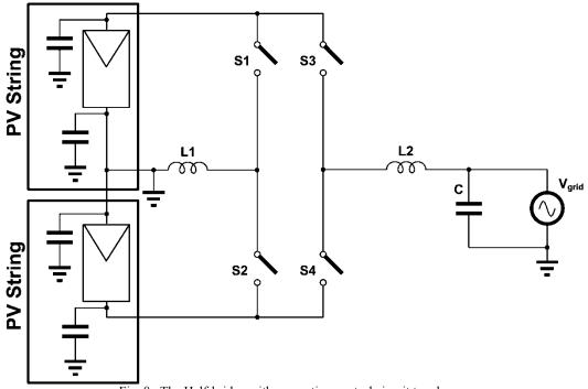
Fig. 8. The Half-bridge with generation control circuit topology.
