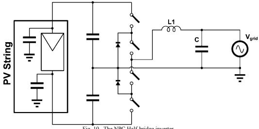
Fig. 10. The NPC Half-bridge inverter.
