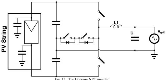
Fig. 13. The Conergy NPC inverter.
