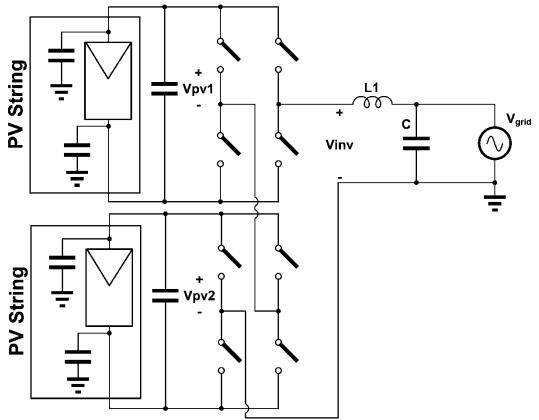
Fig. 9. The cascaded H-bridge multilevel inverter.
