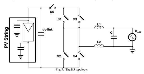
The use of the H5 transformerless inverter topology makes possible to obtain a high efficiency [10], particularly at partial load. It needs only one additional transistor in comparison with the full H-bridge topology. However, as the transistor is in series with the full H-bridge inverter [11], the conduction losses may increase if the semiconductor choice is not optimum.
