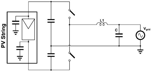
Fig. 5. The Half H-bridge inverter topology.
