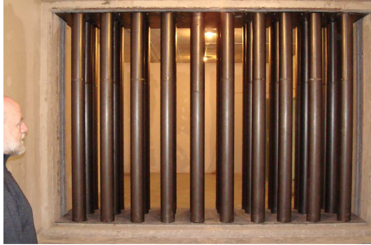
Figure 5.4: Photograph taken inside the transmission chamber. The barrier is schematically described in Fig. 5.2 and has parameters r_1 = r_2 = r_3 = 10 cm, r_{i1} = r_{i2} = 0 , r_{i3} = 4.5 cm, d_1 = 30 cm, d_2 = 50 cm and D = 42 cm.
