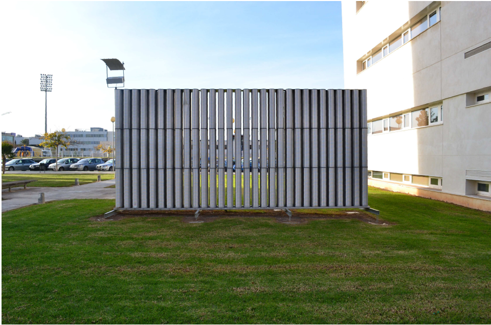
Figure 8.1: Sample made with 3 rows of microperforated 3 m-high cylinders.
