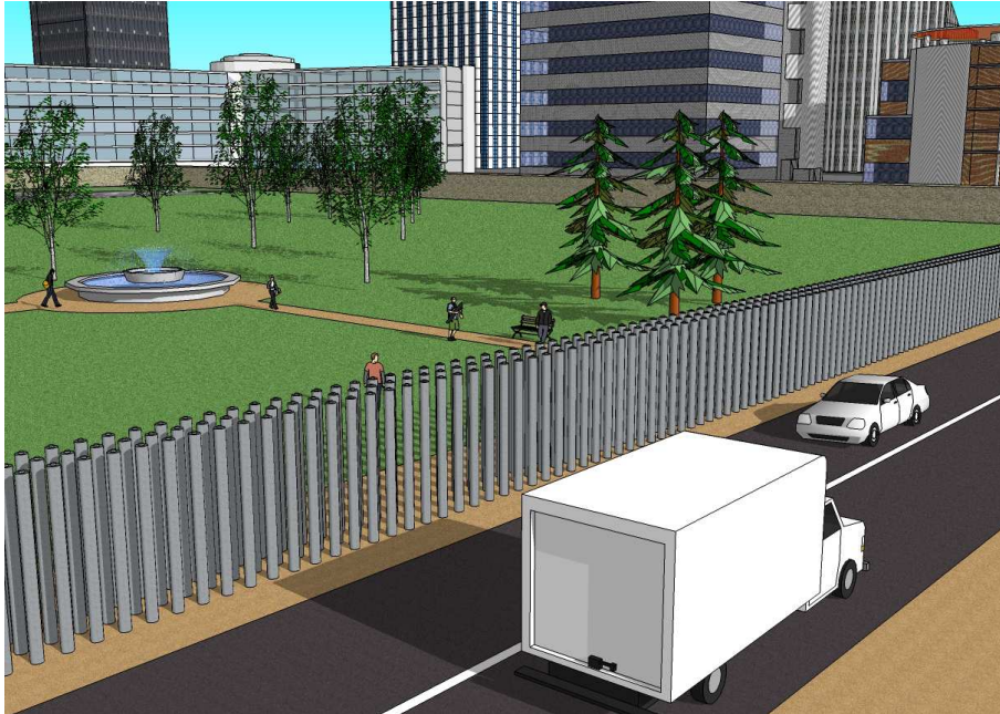
Figure 1.1: Representation of a sound barrier based on a sonic crystal and placed along a road.
