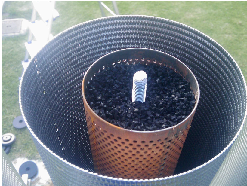
Figure 8.2: Detail of a microperforated shell with radius 8 cm and a porous core of radius 4 cm filled with rubber crumb.
