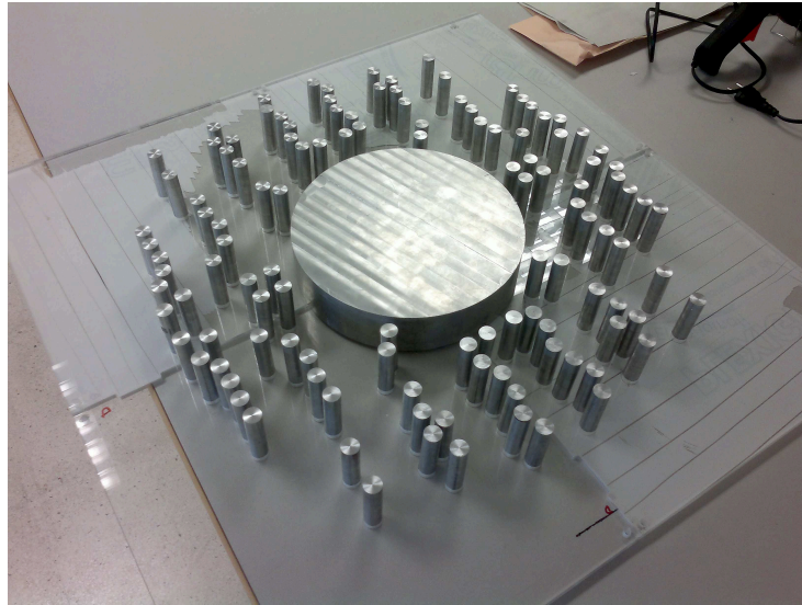
Figure 13.4: Photograph of the fabricated sample consisting of a central cylinder with radius 11.25 cm surrounded by a set of 120 cylinders with 1.5 cm of diameter. All the cylinders are fixed by a methacrylate plate with a distribution of holes drilled in accordance to the scheme of Fig. 13.1.
