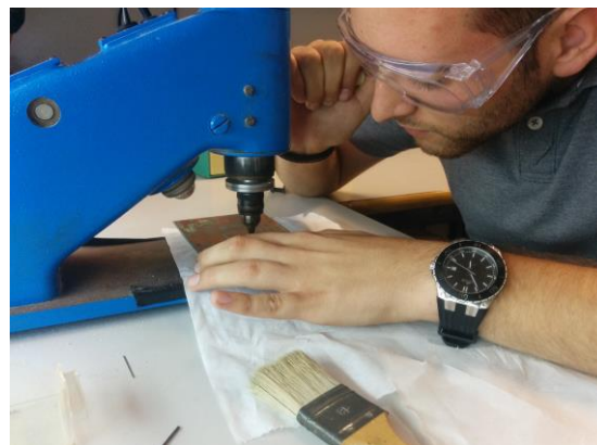
Figure 6-14 – Board being drilled
