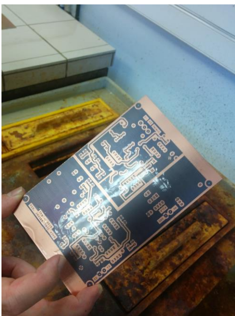
Figure 6-111 – Board after chemical bath
