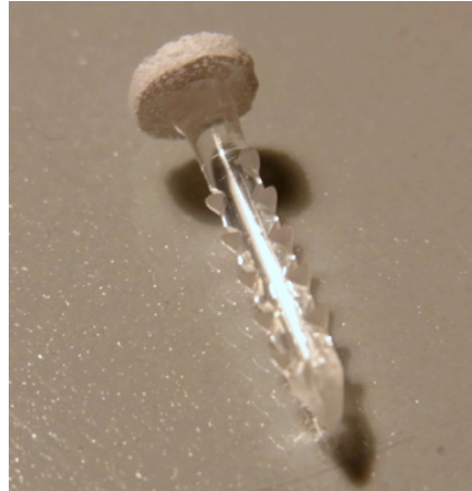
Figure 7.2. The implant device for the second animal trials. The chondral part consists of a porous PCL scaffold and is attached to a PLLA arrow, as anchoring system to the subchondral bone.
