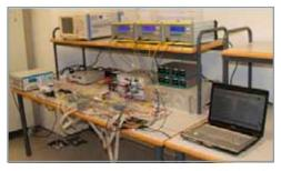
**Figure 9.** Experimental setup assembled in the laboratory to test the feasibility of a two channel subcarrier multiplexed quantum key distribution system
