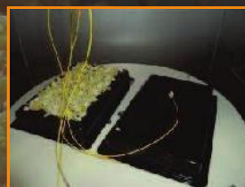
Figure 1. 500g batches of lemon by-product were dried at a frequency of 2450 MHz in an electromagnetic MW generator (Miralbel, France) at a power density of 1.5 watt/g for 60 min.
