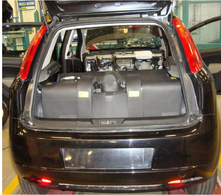
Fig. 7. Picture of the onboard adsorption chiller: (a) in the laboratory and (b) installed in the vehicle.
