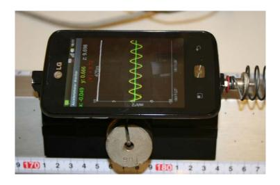
FIG. 2: Photograph of the smart phone displaying a view of the Acceleration Monitor application for the the case of free hammonic oscillations.
